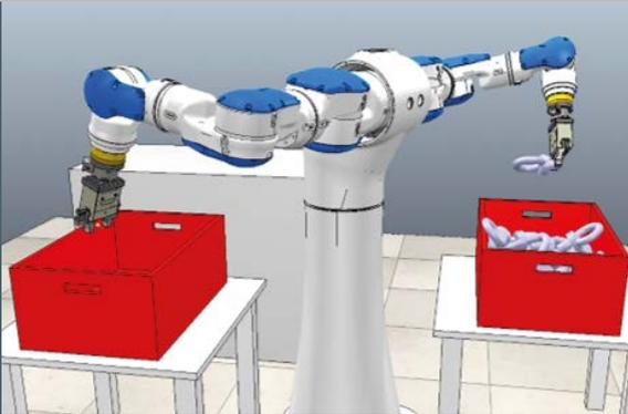
1 Two-armed real and digital twin robot performing a bin picking task.
